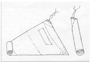
**62.** For storage, roll the jib from the head downwards as shown above, It will then fit into its bag without folding and will unroll, ready for use, without creases. **Never fold the jib across the window.**
